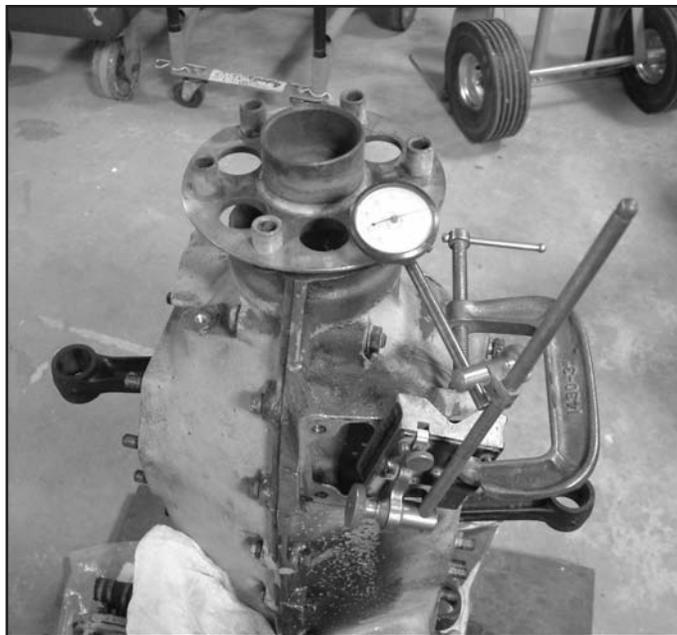
*The first step is to attach the surface plate to a stable surface on the engine. For this example we used a "C" clamp and attached the surface plate to the starter mounting boss, which is cast in the engine case half.*
