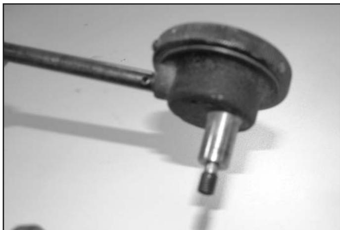
*The sensitive probe which attaches to the dial.*
