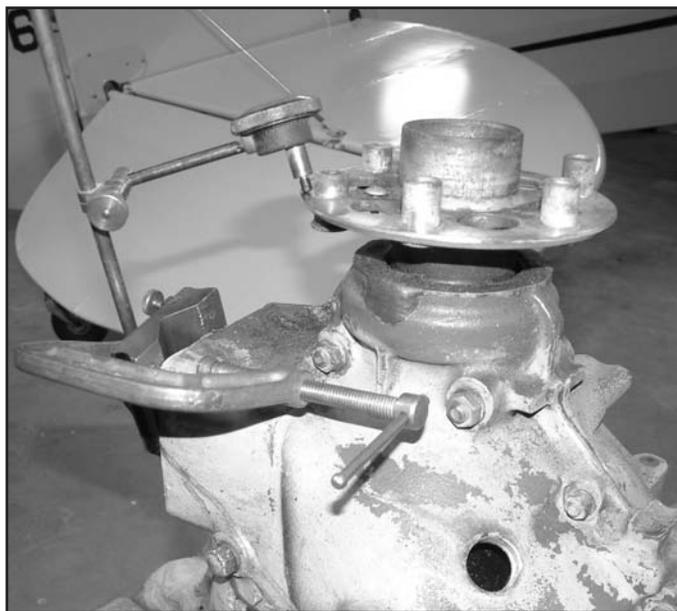
*After firmly attaching the surface plate to the engine, position the indicator arm so that the sensitive probe comes in contact with the outer edge of the prop flange. It must be positioned so that the six flange bushings do not interfere with the probe while rotating the crankshaft.*
